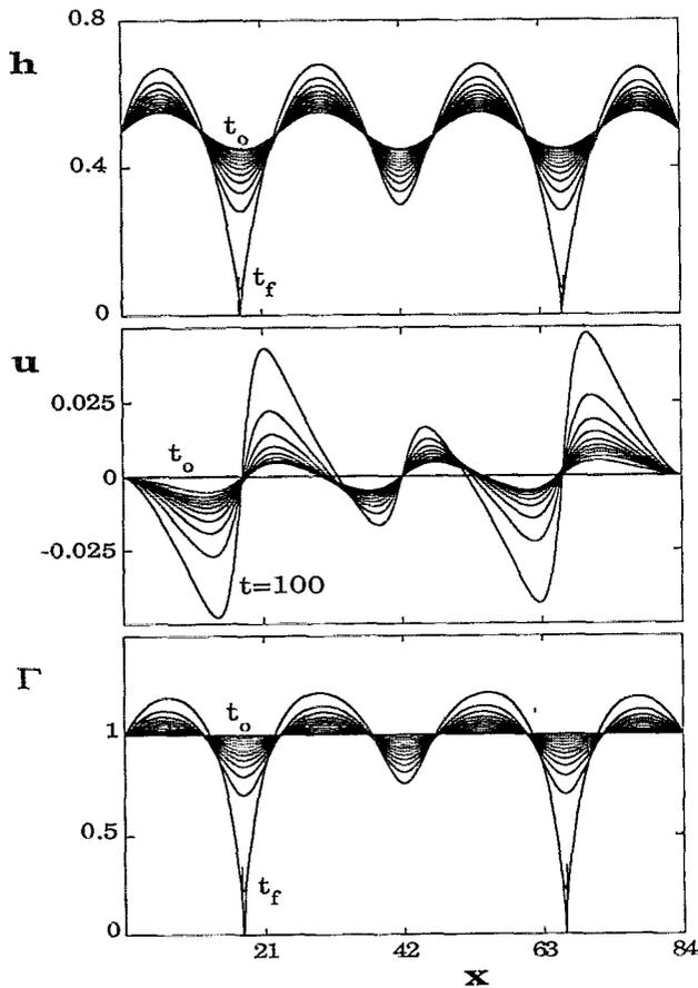
FIG. 7. Rupture of a free film with FBC. All parameters are the same as in Fig. 3 except  $L=84$  and the initial condition is assigned to  $(h, \Gamma, u) = (0.5 + 0.05 \sin[k_m x], 1, 0)$  with  $m=7$  ( $\lambda_i=24$ ). The FBC favor rupture of the film near its edges and as the initial condition is symmetric with regard to the middle of the system, rupture occurs simultaneously at both edges at time  $t_f=110$ .
