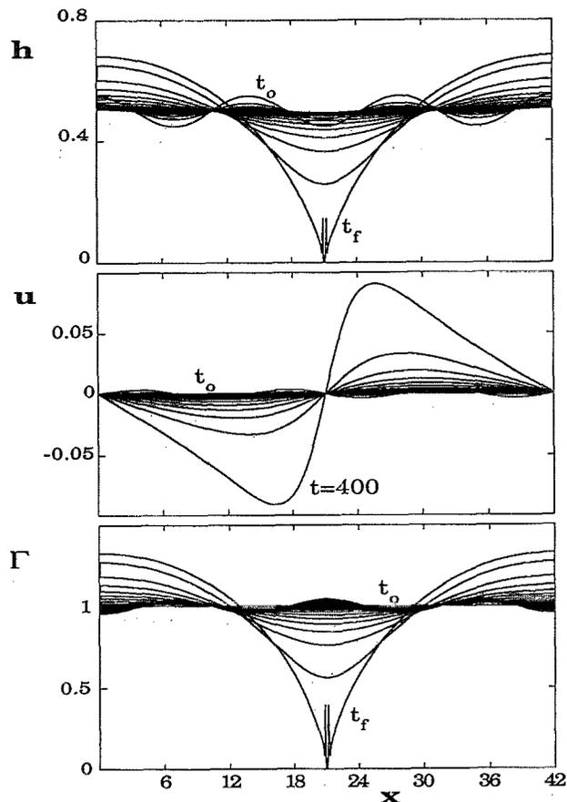
FIG. 6. Rupture of a free film with PBC when the wavelength of the initial disturbance  $\lambda_i$  is smaller than the critical wavelength  $\lambda_c$  but  $L > \lambda_c$ . All the parameters are the same as in Fig. 3 except  $L = 42$ ,  $m = 6$  (hence  $\lambda_i = 14$ ), and  $\Delta t = 20$ . A change of wavelength toward a larger and unstable one occurs, leading finally to the rupture at  $t_f = 407$ .
