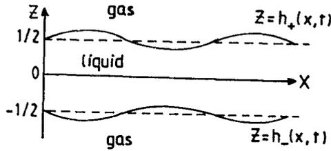
FIG. 1. Sketch of a free film with fluctuating surfaces. The free surfaces are described by the equations  $z = h_{\pm}(x, t)$ . The dashed lines indicate their mean position at  $h = \pm 1/2$ . The squeezing mode, for which the fluctuations of the thickness are symmetric with regard to the axis  $z = 0$ , leads to rupture.
