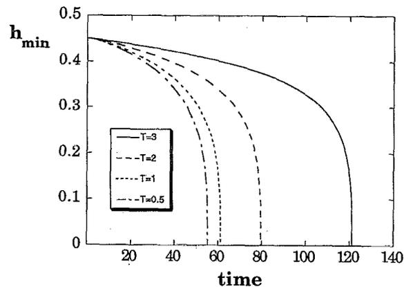
FIG. 4. Minimum of thickness  $h_{\min}$  on the domain  $[0, L]$  plotted as a function of time for different values of  $T$ : 0.5; 1; 2; 3 with  $A=0.05$ ;  $M=0.025$  and  $S_c=10$  on a system  $L=72$  using initial condition of Fig. 3.
