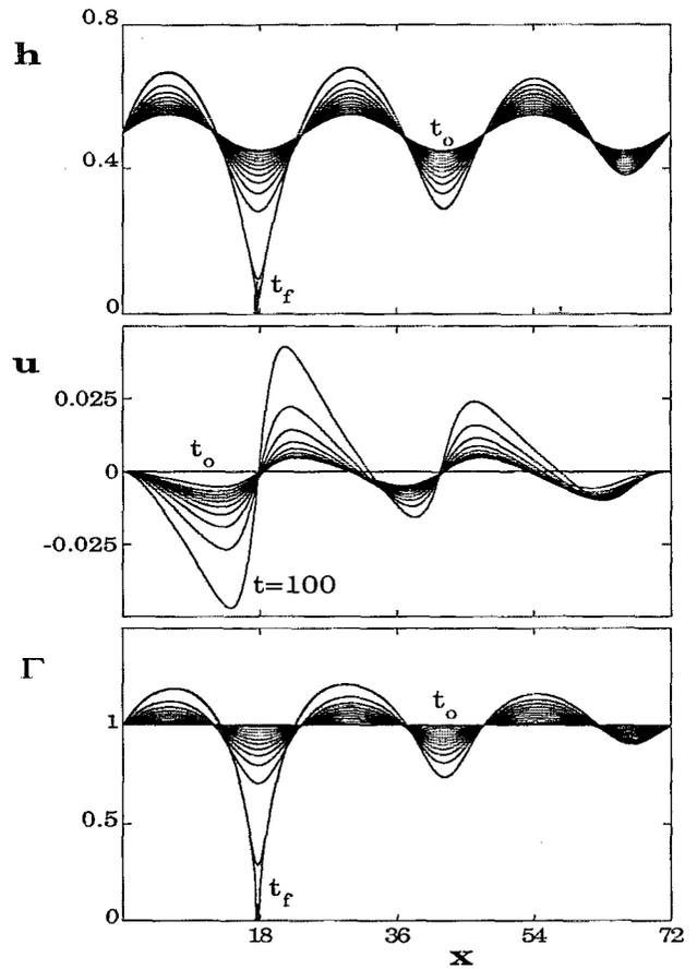
FIG. 8. Rupture of a free film with FBC and the same parameters as in Fig. 6 but  $L=72$  and  $m=6$ . The film is thus asymmetrical with regard to the middle of the system, and rupture occurs only near one edge at  $t_f=110$ .
