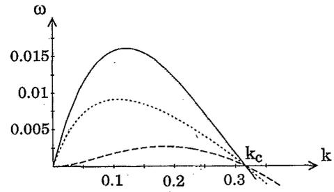
FIG. 2. Growth rate  $\omega$  of the unstable mode versus its wave number  $k$  for increasing values of  $M$ . The straight, dotted, and dashed lines correspond, respectively, to  $M$ : 0.025, 0.05, and 0.1 with  $A=0.05$ ;  $T=3$ ;  $S_c=10$ . The growth rate is positive for all  $k < k_c$ . The variation of  $M$  does not affect  $k_c$  while increasing  $M$  leads to a decrease of  $\omega_{\max}$  and hence to an increase of the rupture time.
