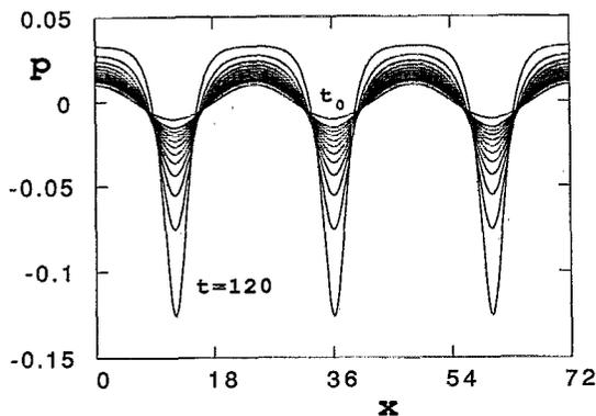
FIG. 5. Variation of the pressure  $p(x,t) = -2u_x - Th_{xx}$  at successive times using PBC and the same initial conditions and parameters  $A$ ,  $T$ , and  $M$ , as in Fig. 3. The pressure is positive in regions of maximum thickness while the pressure is negative in regions of minimum thickness.
